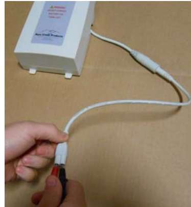
Touch volt meter prongs to the inside of the battery test cable for the Vito battery
