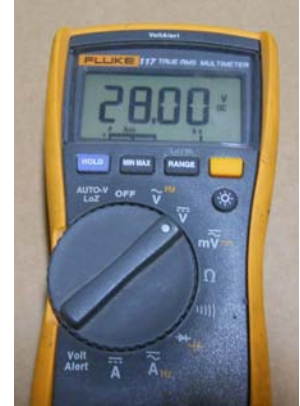
Volt meter should read at least 25.0VDC
