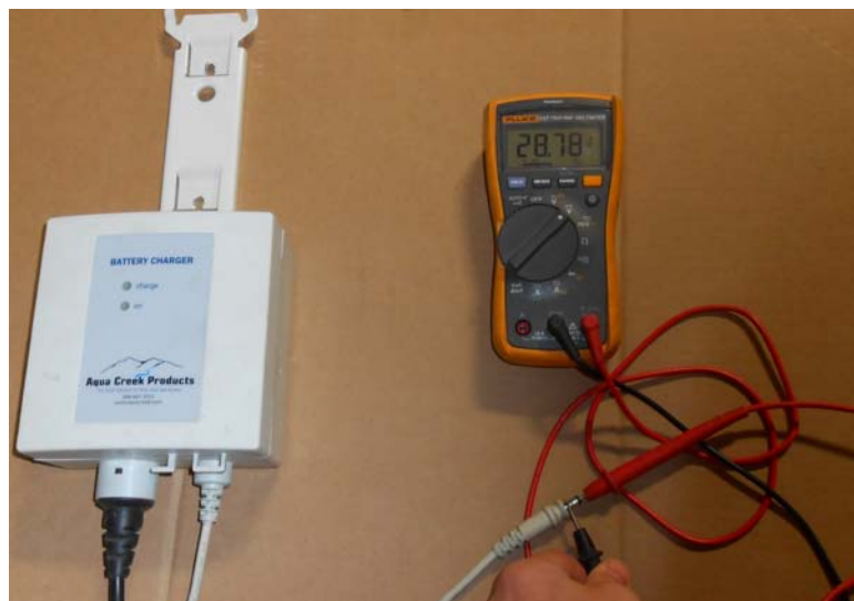
Touch one volt meter prong to the inside of plug and the other to the outside of plug on the Vito charger
