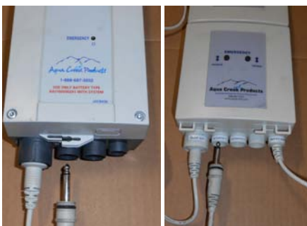
Unplug actuator from Port B and plug in the test light
