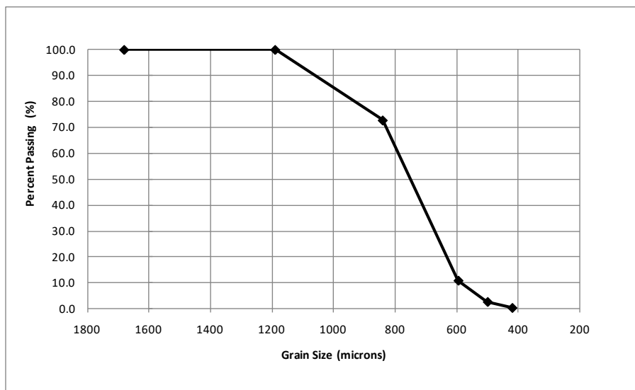
Figure 4.7.2.1.4.2: Grain Size Distribution of Pool Filter Sand – Brand B
