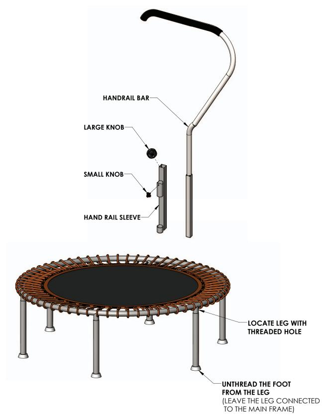
One of the six threaded sockets will have a threaded hole in it. Locate that leg and unthread the rubber foot from the leg. Leave the leg itself attached to the threaded socket. See above.
