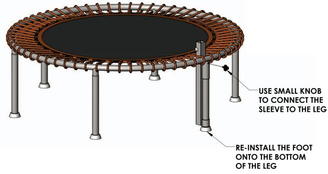
Tighten the sleeve to the leg using the small knob and then re-install the rubber foot to the bottom of the leg. See above.
