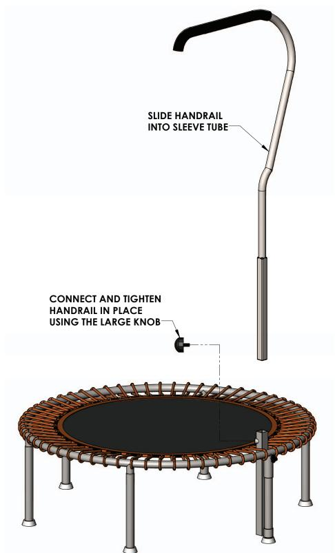
Finally, insert the handrail into the sleeve with top of the handrail angled back towards the trampoline. Lock the handrail in place using the large knob. See above.
