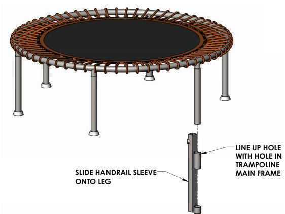
Slide the handrail sleeve onto the leg. Rotate the sleeve so that the hole in the sleeve lines up with the hole in the threaded socket. The square tube should be to the inside of the main frame. See above.
