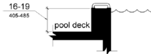
Figure 1009.4.2 Transfer Wall Height
